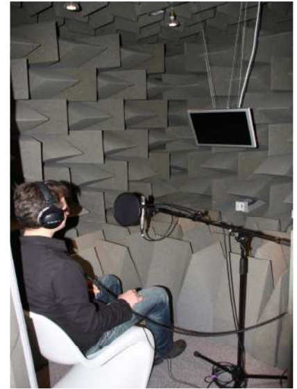
The state-of-the-art anechoic recording studio at the Informatics Forum on Crichton Street, where voice recording takes place
